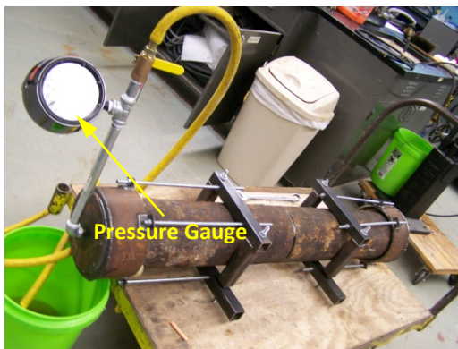
Figure 7: Pressurized leak test performed on the test specimen
