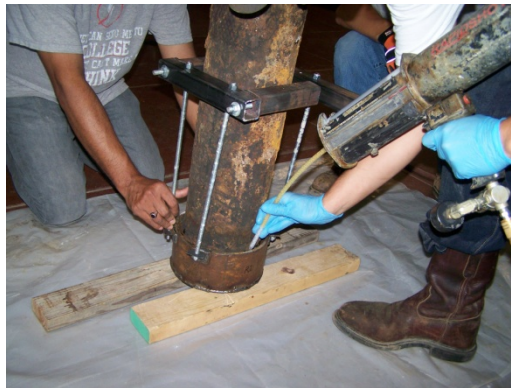
Figure 6: Test specimen hung over the cap (left), application of polyurea (middle) and final setup (right)
