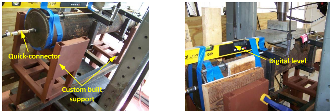
Figure 8: Host pipe placed on custom built support (left) and deflection measurements (right)
