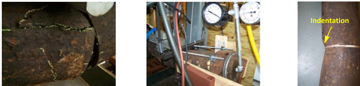
Figure 11: Crushed host-pipe (left); deflected liner holding 120 psi internal pressure (middle); deformation at the liner's crown region (right)
