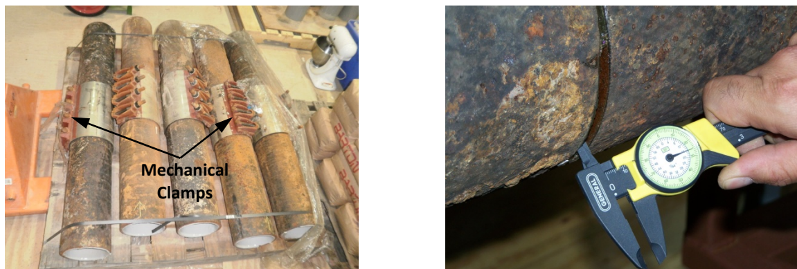
Figure 4: Specimens after lining (left); host-pipe sections after removal of clamps and spacer (right)
