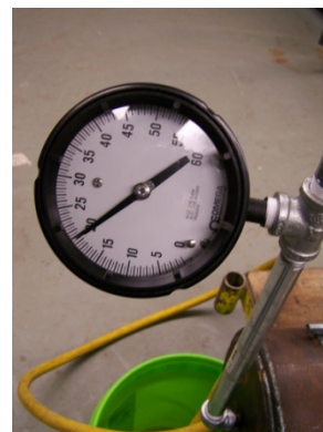
Figure 7: Pressurized leak test performed on the test specimen
