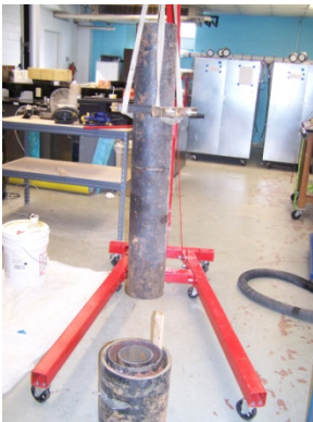
Figure 6: Test specimen hung over the cap (left), application of polyurea (middle) and final setup (right)
