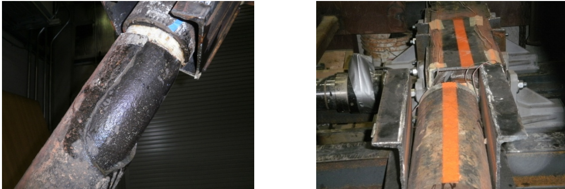
Figure 20: Host-pipe broke at crown-invert plane (left) and 3.5 in. displacement of the liner (right)
