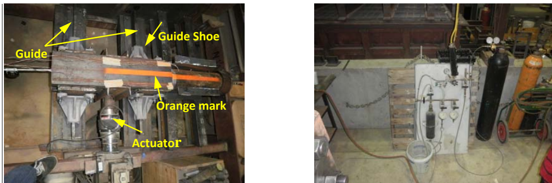
Figure 18: Experimental setup of the shear test (left) and the nitrogen gas operated pressure pump (right)
