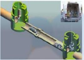
The Plug is inserted into the Sleeve, and Sleeve is centered on the Plug
